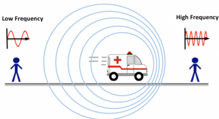
Figure 1. When the source moves toward the listener, the perceived frequency is higher than the emitted frequency, thus
