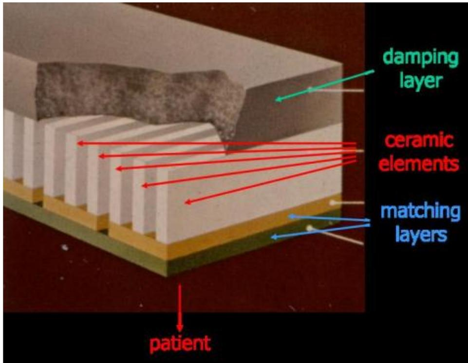
Figure 7. Internal parts of a transducer.
